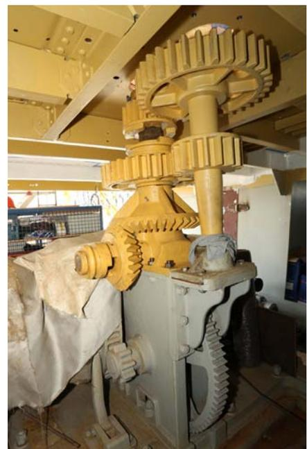
Gearpill mechanism in the forepeak in the bow of the PEKING
