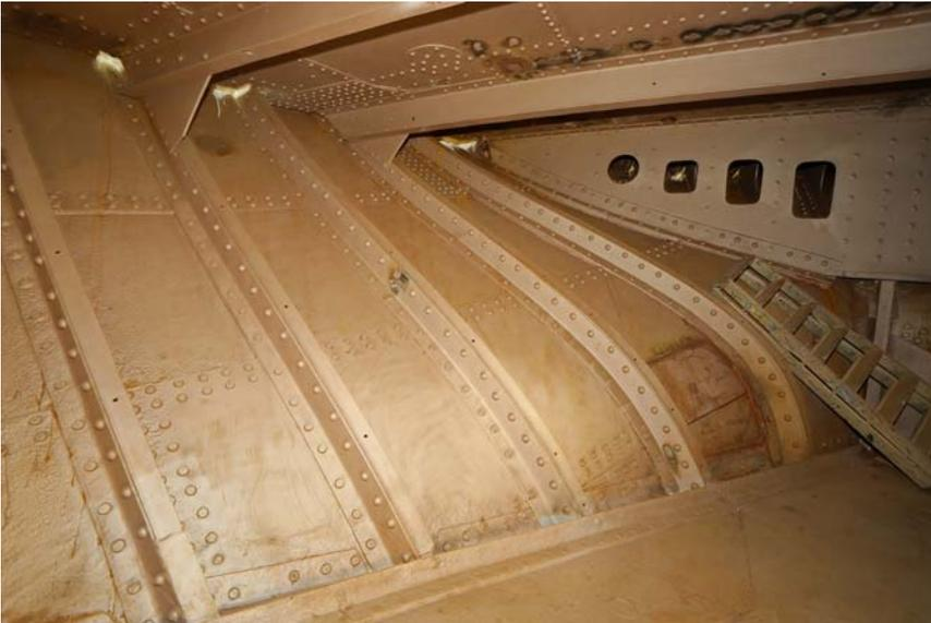
Frames and riveted hull in the stern of the ship at tweendeck level
